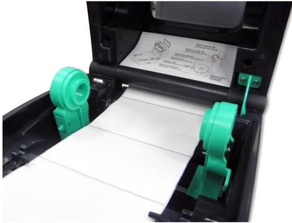
4. Feeds the media through the rear external label entrance chute. And place the paper, printing side face up, through the media sensor and place the label leading edge onto the platen roller. Move the media guides to fit the label width by turning the guide adjuster knob.
