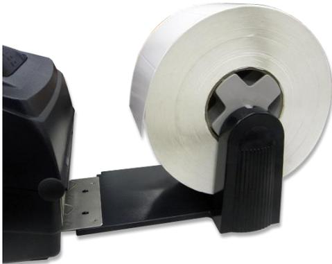
2. Insert a 3" label spindle into a paper roll. And install it on the external paper roll mount.
