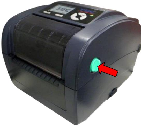
1. Open the printer top cover by pulling the tabs located on each side towards the front of the printer then lift the top cover to the maximum open angle.
