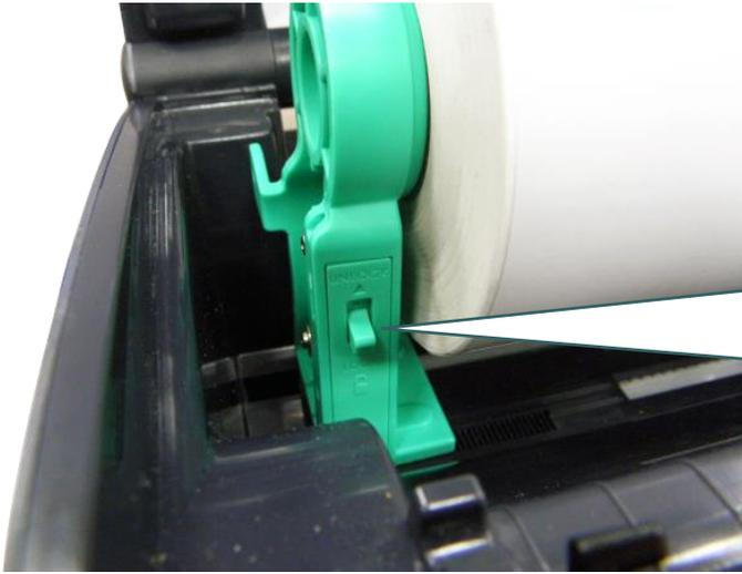
4. Press down the media holder lock switch to hold the label roll firmly.
