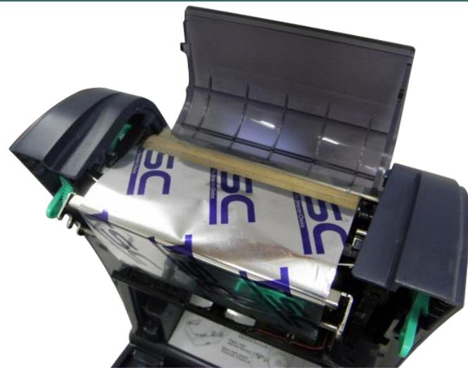
5. Stick the ribbon onto the ribbon rewind paper core.
