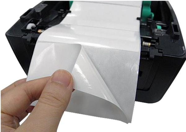
3. Open the printer cover. Pull the label through the front of the printer and take some labels off only leave the liner.
