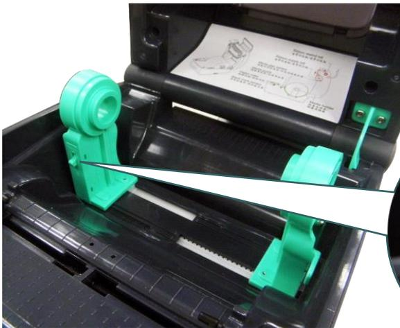
3. Open the printer's top cover and separate the media holders to fit the media width. Press down the media holder lock switch to fix the media holder.
