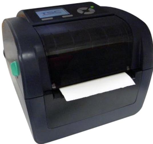
6. Disengage the top cover support and close the top cover gently.
