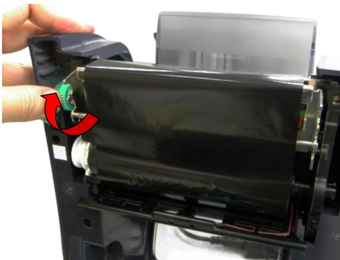
6. Turn the ribbon rewind gear until the ribbon plastic leader is thoroughly wound and the black section of the ribbon covers the print head.
