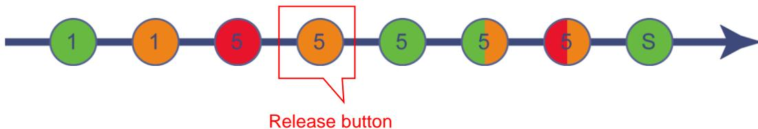
4. It calibrates the sensor and measures the label length and prints internal settings then enter the dump mode.
