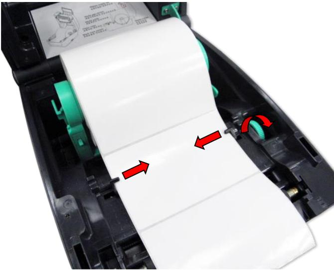
5. Place the paper, printing side face up, through the media sensor and place the label leading edge onto the platen roller. Move the media guides to fit the label width by turning the guide adjuster knob.
