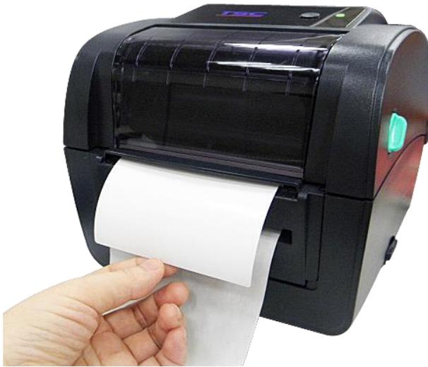
6. Disengage the top cover support to close the top cover. Printer is ready for peel-off mode.
