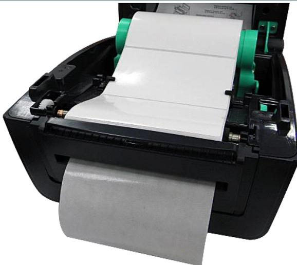
5. Close the peel-off module. Use the DiagTool or LCD menu function to enable the peel-off mode.
