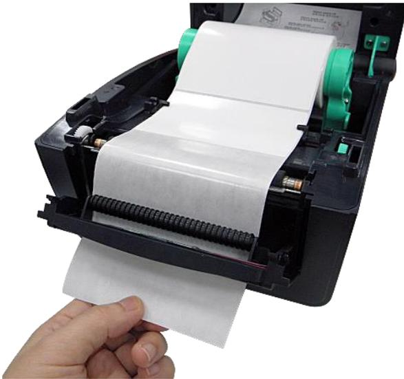
4. Open the peel-off module cover. Feed the liner into peel-off cover slot.
